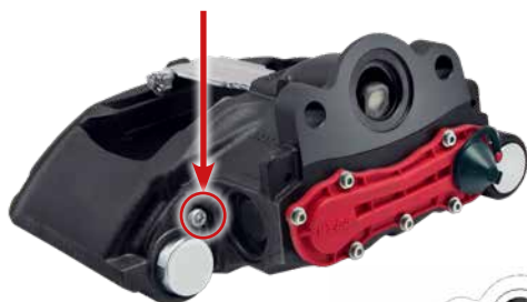
MC225 - two visible bolts near short and long guide sleeve ports
