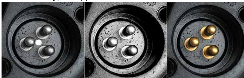
On/Off Sensor: Silver colored pins and white dot in middle
