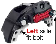
Left side fit bolt Part #: BR4700-43 Right long guide sleeve
